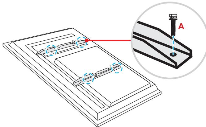
**Note:** Dual mounting brackets, wall mount, and screws (A) are included in the wall mount kit. Refer to “Wall Mounting Installation” on page 12.
