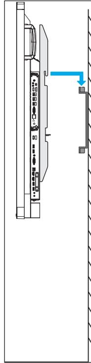
5. Secure the dual mounting brackets and the wall mount with two screws (C).
