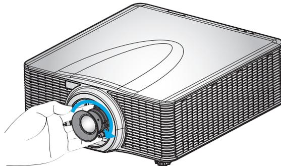
5. Firmly install the lens ring onto the lens.
