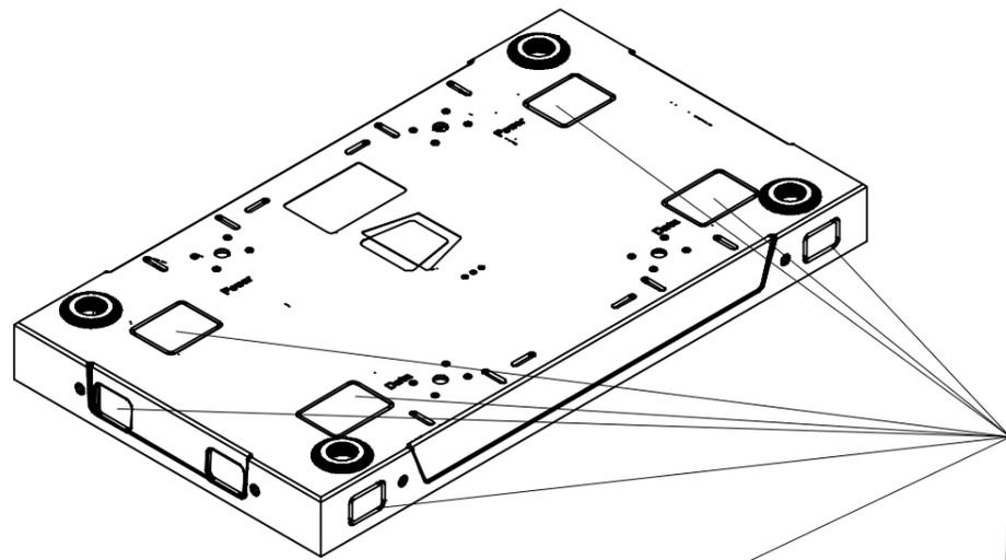
COPPER FOIL CABLE PASS THROUGH APERTURE POINTS
